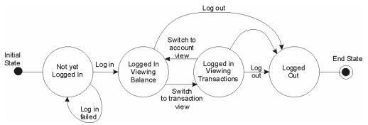
The initial state is where the state machine starts (the circle marked Initial state, and the one marked End State are not states themselves – rather pointers to the actual initial and end states). Each state is represented by a circle. Each arrow represents a message that can be received by the state machine (often triggered by an event) that can cause the machine to change states. Thus in this example, a successful log-in moves the application into the account viewing state.
